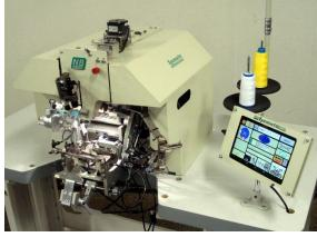
Electronic Button/Counter Button Sewer & Neck Wrapper
